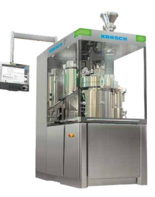
Offering a 100kN pre and main compression capability, a maximum press speed of 120 RPM, and an extended feeder length, the SFP is geared for high-speed production, with a maximum output of 338,400 tablets per hour. An ergonomic and accessible design permits the fastest changeover of any machine in its class.
